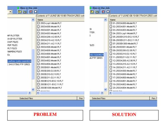
Using this technique, you could combine all pages for a project (A, S, MEP) in one folder, and using a two or three digit number to guarantee page position in that set. Often an architect has pages in a set which do not have an A as a page number (life safety, demo, noas, etc) but need to be included with the architecturals. A simple renaming when creating PLT files would relieve much of the uncertainty and insure job correctness.
